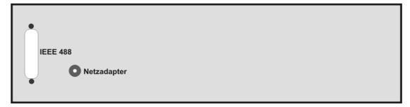
The rear panel contains the charger jack and the data bus connector.
