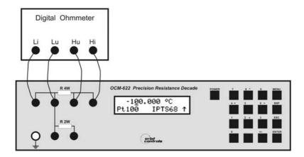
Recommended schematic for R27 to R35 (Terminals R2W)
